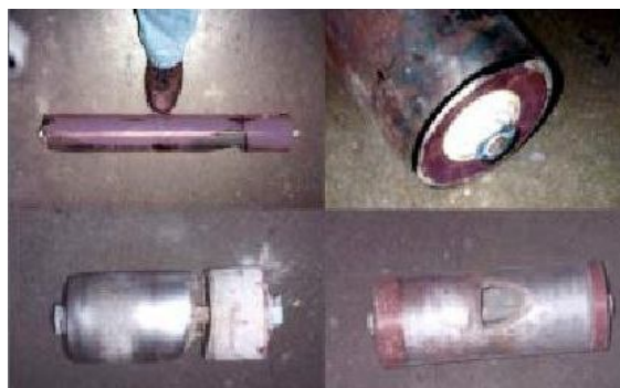
Fig.4 Failure of rollers
